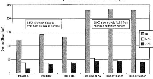
3M™ Thermally Conductive Adhesive Transfer Tapes
