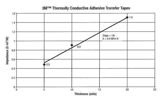
Thermal Impedance (C-in²/W) vs. Thickness: (Test Conditions: 3M test method).
